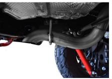
To install your XT Tip simply remove the exhaust from the Gibson head pipe and re install the tip using the same clamp and driver side only hanger. Protect your tips when in storage. We do not want any dings or dents
