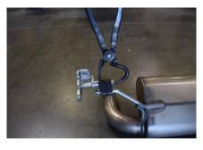
Remove hangers from OEM exhaust using removal pliers or large channel pliers and re-install them on the Gibson as shown. Using a lubricant can aid in the removal.
