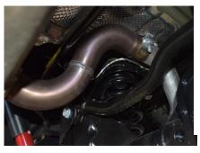
3. Once you have removed the OEM exhaust install Item# E onto the factory oem pipe. Use clamp # b to secure. Be sure notch is lined up and do no tighten clamp.
