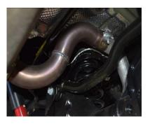
3. Once you have removed the OEM exhaust install Item# E onto the factory oem pipe. Use clamp # b to secure. Be sure notch is lined up and do no tighten clamp.
