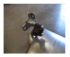
2.Remove the factory exhaust hangers from the using a 13 mm removing the two bolts. These hangers will remain attached to factory muffler when being removed.
