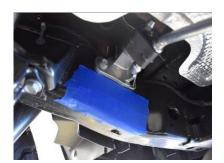
5. Slide the second supplied 2.5" band clamp over the headpipe then slip your new Gibson muffler onto the headpipe, tighten aluminum hangers into their locations with the 4 factory bolts.
