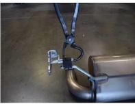
4. Remove hangers from OEM exhaust using removal pliers or large channel pliers and re-install them on the Gibson as shown. Using a lubricant can aid in the removal.
