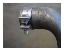
1.Be sure to check all parts are correct and match the Manual. Loosen the factory OEM clamp located just in front of the muffler above the factory axle. This will require a 15MM.
