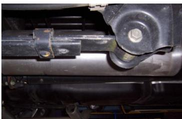
INSTALL MUFFLER #B ONTO HEAD PIPE 1-1/2" TO 2" WITH THE LOUVERS FACING TOWARDS THE CONVERTER. THE MUFFLER OUTLET SHOULD BE POSITIONED THE MUFFLER OUTLET SHOULD BE POSITIONED AT 12:00. USE A JACK STAND TO SUPPORT THE MUFFLER. USE CLAMP #E TO SECURE THE MUFFLER TO THE HEAD PIPE. DO NOT TIGHTEN. MUFFLER INLET IS LOOKING INTO THE LOUVERS.
