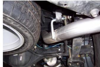
INSTALL THE OVERAXELE TAILPIPE #C INTO THE MUFFLER 1-1/2" TO 2". INSERT WELDED HANGERS INTO RUBBER GROMMET. SECURE TO THE MUFFLER USING CLAMP #E. DO NOT TIGHTEN.
