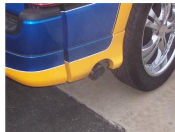
NEXT INSTALL YOUR STAINLESS STEEL TIP TO YOUR DESIRED LOOK. USE ANY ALUMINUM OR STAINLESS STEEL CLEANER TO POLISH YOUR TIP. MAKE SURE YOU HAVE A MINIMUM OF A 1" CLEARANCE ON ALL PIPES FROM ALL RUBBER BRAKE LINES, TIRES, SHOCKS, FUEL LINES, ETC. THEN TIGHTEN ALL CLAMPS AND HANGERS
