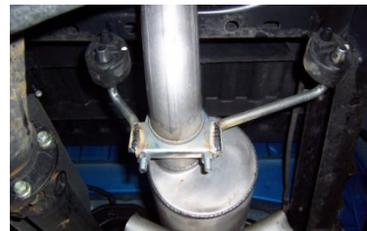
NEXT INSTALL REAR MUFFLER HANGER #G ONTO OUTLET OF MUFFLER. INSERT WELDED HANGER INTO RUBBER GROMMETS
