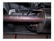
2. To remove your stock exhaust, measure and cut 8" in front of the muffler. Disengage the welded hangers from the OEM rubber grommets. Use WD-40 to aid in this process. Do not damage or remove the rubber grommets as you will reuse them to mount your new system. Now, cut off tailpipe and remove exhaust.
