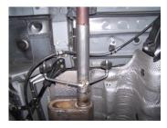
3. Install headpipe #A onto your existing stock front pipe and attach with clamp #E. Use a jack stand to support the converter. Insert welded hangers into rubber grommets.
