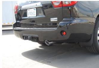
7. Install stainless steel tip. Clamp down. When you have everything in place, firmly tighten all bolts and clamps down securely. Use stainless steel cleaner and a Scotch Brite pad weekly to prevent tip from discoloration. Inspect all fasteners after 25-50 miles of operation and re-tighten as necessary. You may need to cut your stock tail pipe back to get your tip to fit correctly.
