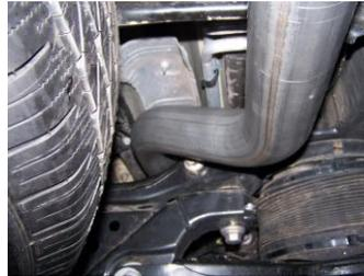
6. Install the overaxle tailpipe #E to the rear extension pipe #D. Use clamp #H to secure pipe. Do not tighten. Install welded hanger into rubber grommet.
