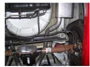
6. Now install the passenger side muffler assembly #C by sliding the metal hangers into the rubber grommets. Then do the same for the driver side muffler assembly #D.
