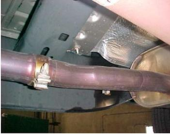
TO REMOVE YOUR STOCK EXHAUST, REMOVE IT FROM THE CLAMP LOCATED JUST IN FRONT OF THE MUFFLER AND REMOVE HANGERS FROM RUBBER GROMMETS BY PULLING EXHAUST TOWARDS THE REAR OF THE VEHICLE, USE WD-40 TO AID IN REMOVAL, LEAVE GROMMETS IN PLACE.
