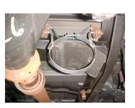
Install band clamp # G into rubber grommets located just above the axle. Do not tighten. And attach with bolt kit # H.
