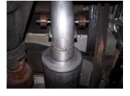
11. Slide the over axle tailpipe #C into muffler 11/2"-2". Use clamp #F to secure. Do not tighten. Insert welded hangers into rubber grommets.
