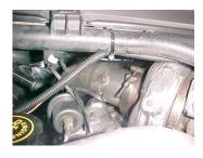
4. Remove the remaining stock downpipe by unclamping it from the turbo housing. Use an 11mm socket or wrench to remove your stock pipe through the bottom. Do not discard the stock you will need to reuse it. Now, install downpipe #A onto turbo reusing your stock clamp. Do not tighten.
