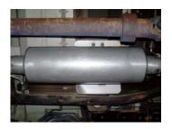
8. Install muffler #B onto head pipe 11/2"-2". Use a jack stand to support the muffler. Use clamp #F to secure the muffler to the headpipe. Do not tighten.
