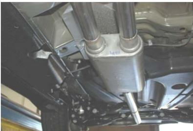
4. Install muffler #B onto headpipes #A 1.5-2" with the louvers facing towards the converter. Use a jack stand to support the muffler. Use clamp #G to secure the muffler to the headpipes. Do not tighten. Muffler inlet is looking into the louvers.
