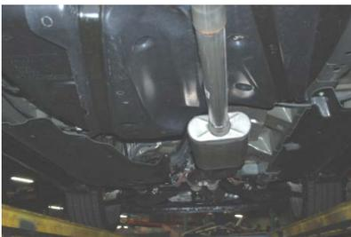
5. Install extension pipe #C onto muffler outlet. Use clamp #H to secure the pipe to the muffler.
