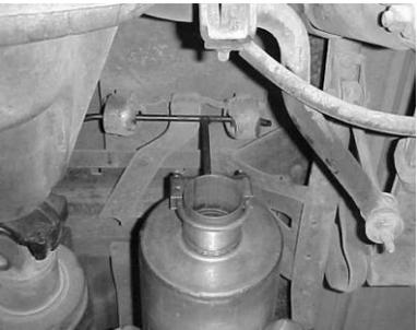
4. Slide muffler # B with inside louvers facing towards the converter. Use a jack stand to support the muffler. Install hanger # G on the muffler outlet. The long portion of the hanger will be pointing towards the driver side. Now, install rear hanger # H with hanger bolts facing towards the passenger side. Install over axle pipe # C into the outlet of muffler no less than 1 1/2" and no more than 2". Do not tighten hangers.
