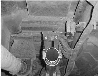
3. Install headpipe # A. **SHORT BEDS:** You may need to cut head pipe # A to length on short bed models. Use clamp # F to attach head pipe to factory connector pipe. Install hanger # I at the rear of the head pipe using supplied nuts and bolts. Do not tighten.
