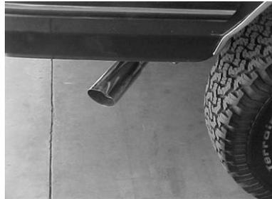
6. Install stainless steel tip, Clamp down. To clean stainless tip use any stainless steel or aluminum cleaner. When you have everything in place, make sure you have a 1" clearance on all pipes from all rubber brake lines, shock boots, tires, etc. Tighten all bolts and clamp down.
