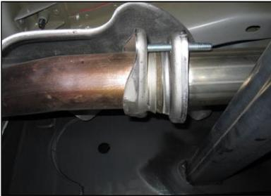
INSTALL HEADPIPE # A INTO STOCK PIPE. USING BOLT KIT PROVIDED INSERT WELDED HANGERS INTO RUBBER GROMMET.. DO NOT TIGHTEN.
