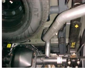
INSTALL OVERAXLE TAILPIPE #C INTO MUFFLER 1 1/2" TO 2". INSERT HANGERS INTO RUBBER GROMMETS. USE CLAMP #E TO SECURE PIPE TO MUFFLER. DO NOT TIGHTEN.
