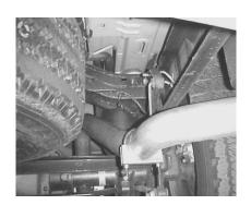
INSTALL EXIT PIPE #D AND ATTACH TO TAILPIPE WITH CLAMP #F. DO NOT TIGHTEN. ROTATE OVERAXLE PIPE AND TURN OUT PIPE UNTIL IT BEST FITS YOUR VEHICLE.
