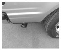
INSTALL STAINLESS STEEL TIP. USE ANY ALUMINUM OR STAINLESS STEEL CLEANER TO POLISH YOUR TIP. NOW FIRMLY TIGHTEN ALL CLAMPS AND HANGERS.
