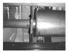
DO NOT REMOVE EXTENSION PIPE BETWEEN MUFFLER AND CATALYTIC CONVERTER.
