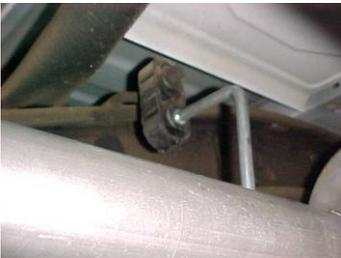
Install the driver side over axle tailpipe # D into the muffler 1-1/2" to 2". Use clamp # H to secure to the muffler. Do not tighten. Use clamp # I into to hold up the hanger. Do not tighten.
