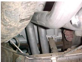
**MAKE SURE YOU HAVE A 1" CLEARANCE ON ALL RUBBER BRAKE LINES, SHOCK BOOTS, FUEL LINES, TIRES, ETC..**
