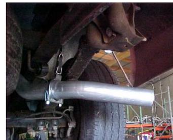
Install muffler # B on to head pipe 1-1/2" to 2" with the louvers facing towards the converter. Use a jack stand to support the muffler. Use clamp #G to secure the muffler to the head pipe. Do not tighten.
