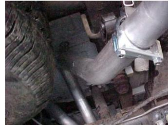
Install the passenger side over axle tailpipe # C to the muffler 1-1/2" to 2". Use clamp # I to secure tailpipe to muffler.
