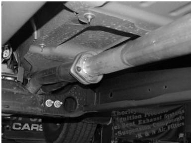
BOLT HEADPIPE #A TO STOCK FLANGE RE-USING FACTORY NUTS. DO NOT TIGHTEN AND CONNCT WITH CLAMP #F. SLIDE WELDED HANGER INTO RUBBER GROMMET. INSTALL HEAD PIPE EXTENSION #J.
