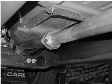
BOLT HEADPIPE #A TO STOCK FLANGE RE-USING FACTORY NUTS. DO NOT TIGHTEN AND CONNECT WITH CLAMP #F. SLIDE WELDED HANGER INTO RUBBER GROMMET. INSTALL HEAD PIPE EXTENSION #J.
