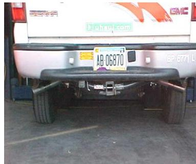
INSTALL EXIT PIPES #E ONTO TAILPIPES AND ATTACH TO HANGER #H AND CLAMP #G TO SECURE EXIT PIPES TO TAILPIPES. THESE METAL HANGERS NEED TO BE ROTATED IN ORDER TO ADJUST FOR CLAMPING. CUT TO YOUR PREFERRED LENGTH. NOW INSTALL YOUR STAINLESS STEEL TIPS TO YOUR DESIRED LOOK. NOW YOU CAN TIGHTEN ALL CLAMPS, NUTS, AND BOLTS. STARTING FROM THE FRONT WORKING BACK. USE ZIP TIES TO TIE AWAY BRAKE LINES.
