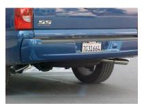
INSTALL EXIT PIPES # F ONTO TAILPIPES. CUT TO YOUR PREFERED LENGTH USE CLAMPS # I TO SECURE EXIT PIPES TO TAILPIPES. THESE CLAMPS ALSO ATTACH TO METAL HANGERS # J. THESE METAL HANGERS NEED TO BE ROTATED IN ORDER TO ADJUST FOR CLAMPING. ROTATE EXIT PIPES TO POINT OUT TO THE SIDE. NOW YOU CAN TIGHTEN ALL CLAMPS, NUTS, AND BOLTS. STARTING FROM THE FRONT WORKING BACK. INSTALL STAINLESS TIPS. USE ZIP TIES FOR BRAKE AND FUEL LINES
