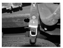
INSTALL METAL HANGERS # J INTO SLOTTED HOLES LOCATED APPROX. 16" FROM THE REAR OF THE FRAME. METAL HANGERS ARE MOUNTED ON THE OUTSIDE OF FRAME. USE THE HARDWARE THE PROVIDED. THE BOLT AND WASHER WILL GO INTO THE 1ST HOLE FROM THE TOP OF THE HANGER.
