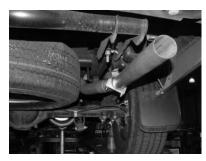
INSTALL PASSENGER SIDE TAILPIPE #C INTO MUFFLER AT LEAST 1 ½" TO 2". USE CLAMP # I TO SECURE PIPE TO MUFFLER. DO NOT TIGHTEN. THE TAILPIPES WILL BOTH LEAN TOWARDS THE DRIVER SIDE FOR CLEARANCE. LOOKING FROM THE REAR OF THE VEHICLE – THIS TAILPIPE IS AT APPX. 11 O'CLOCK.
