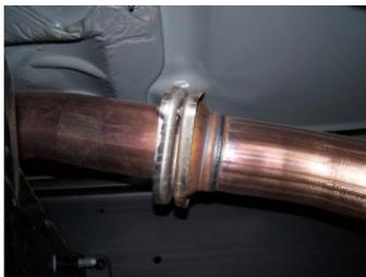
2. To remove the stock exhaust, unbolt the head pipe at the 2 bolt flange. Disengage the welded hangers using WD-40 from the OEM rubber grommets. Do not damage or remove the rubber grommets as you will reuse them to mount your new system.
