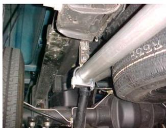
9. Install tail pipe hangers #H onto end of tail pipes using clamp #G. There will be about a 2" hole above the end of both tail pipes on the frame to bolt the hangers. Do not tighten.
