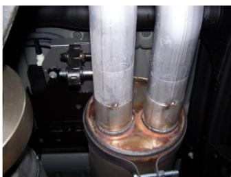
4. Slide muffler #B onto head pipe #A 1 1/2"-2" with the louvers facing towards the converter. Use a jack stand to support the muffler. Use clamp #I to secure the muffler to the head pipe. Do not tighten. Install band clamp #J onto muffler. Insert hanger on band clamp into rubber grommets. Use bolt kit provided. Do not tighten.
