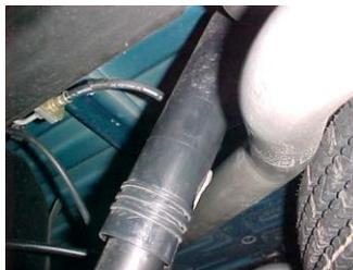
7. Install driver side over axle tail pipe #D into muffler 1 1/2"-2". Support end of tail pipe with jack stand and attach to clamp #G.
