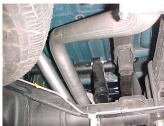
8. Install passenger side over axle tail pipe #C into muffler 1 1/2"-2". Secure with clamp #G. Do not tighten.
