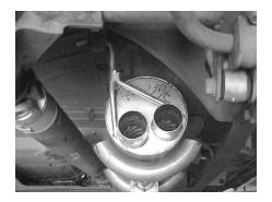
Install muffler # B with the inlet towards the converter onto the head pipe at least 1-1/2" to 2" using clamps #F. Use a jackstand to support. The inlet of the muffler should be at about 6'oclock.Do not tighten.
