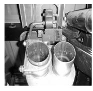
MAKE SURE YOU HAVE A 1" CLEARANCE FROM SHOCKS, SPARE TIRE, PIPES, BRAKE LINES, FUEL LINES, ETC...
