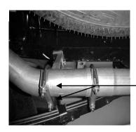
INSTALL HANGER #G ON TAILPIPES AND ATTACH CLAMP #I TO TAILPIPE. ATTACH EXIT PIPES WITH CLAMP #I TO THE TAILPIPES.
