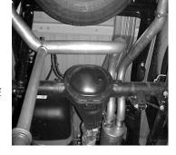
INSTALL OVERAXLE PASSENGER TAILPIPE #E TO OUTLET OF MUFFLER WITH CLAMP #I. SPARE TIRE MAY NEED TO BE LOOSENED AND PUSHED TO THE REAR OF THE TRUCK FOR CLEARANCE PURPOSES.. INSTALL DRIVER SIDE OVERAXLE TAILPIPE #C AND #D, AND CLAMP DOWN HANGER #H TO MUFFLER & TAILPIPE. USE CLAMP #I TO CONNECT BOTH PIPES. DO NOT TIGHTEN!
