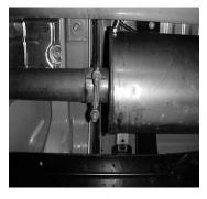
DO NOT REMOVE THE FACTORY EXTENSION PIPE BETWEEN THE MUFFLER AND THE CONVERTER.
