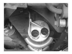
Install muffler #B with the inlet towards the converter onto the head pipes at least 1-1/2" to 2" using clamps #F. Use a jackstand to support. The outlets of the muffler should be at the 6 o'clock position.
