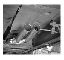
Bolt head pipe #A to the stock head pipe flange behind the converter reusing stock bolts and supplied gasket #I. Use a Hi-Temperature 02 sensor safe silicone on the gasket for a good seal. Insert welded hanger on driver side into rubber grommet. Re-install 02 sensor into head pipe. Apply a small amount of anti-seize on the threads. Do not tighten.
