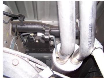
SLIDE DRIVERS SIDE TAILPIPE #D INTO MUFFLER 1-1/2" TO 2". INSERT WELDED HANGER INTO RUBBER GROMMET.
