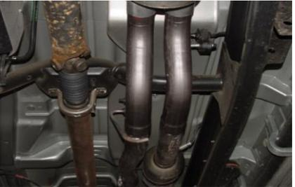
SLIDE PASSENGER SIDE HEADPIPE #A ONTO STOCK HEADPIPE. INSERT WELDED HANGER INTO RUBBER GROMMET. NEXT INSTALL DRIVERS SIDE HEADPIPE #B ONTO STOCK HEADPIPE, USE CLAMP #H TO SECURE BOTH HEADPIPES, DO NOT TIGHTEN.
