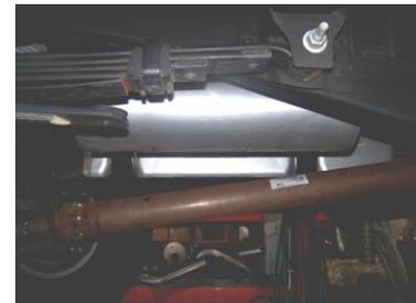
SLIDE MUFFLER #C ONTO HEADPIPES 1-1/2" TO 2". OUTLETS SHOULD BE AT THE BOTTOM. USE A JACK STAND TO SUPPORT MUFFLER.
