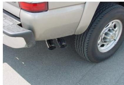
INSTALL YOUR STAINLESS STEEL TIPS. TO CLEAN TIPS USE A SCOTCH BRITE PAD AND ANY STAINLESS OR ALUMINUM CLEANER. AFTER YOU HAVE CHECKED FOR CLEARANCES GO BACK AND TIGHTEN ALL NUTS, BOLTS AND CLAMPS.
