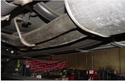
TO REMOVE STOCK EXHAUST, CUT 13" FROM THE FRONT OF THE MUFFLER, MEASURE TOWARDS THE FRONT OF THE VEHICLE. LEAVE ALL RUBBER GROMMETS ON THE HANGERS. USE WD-40 TO AID IN THE REMOVAL OF EXHAUST AND HANGERS. SUPPORT THE CATALYTIC CONVERTER BEFORE CUTTING.
