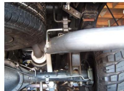
SLIDE PASSENGER SIDE TAILPIPE #E INTO MUFFLER 1-1/2" TO 2". USE CLAMP #I TO SECURE TAILPIPE TO MUFFLER. DO NOT TIGHTEN. INSERT HANGER INTO RUBBER GROMMET.
