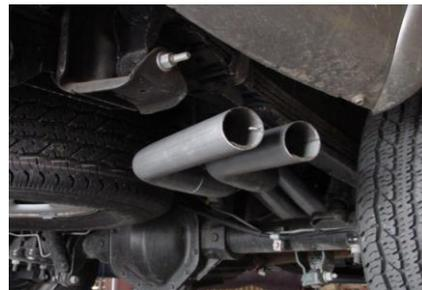
USE BOLT KIT #J TO SECURE TAILPIPES TOGETHER. THE PASSENGER SIDE TAILPIPE WILL BE ON THE BOTTOM.
