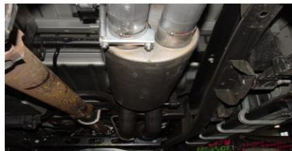
SLIDE MUFFLER #C ONTO HEADPIPES 1-1/2" TO 2". OUTLETS SHOULD BE AT THE BOTTOM. USE A JACK STAND TO SUPPORT MUFFLER.
