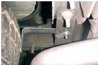
INSTALL SPARE TIRE BRACKET #K ONTO HOLE IN FRAME LOCATED ABOVE TAILPIPE HANGER. HOLE IS ABOUT 1" ROUND.
