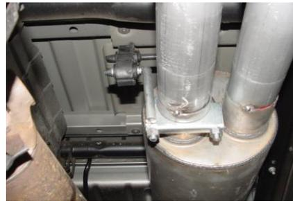
INSTALL HANGER #H INTO RUBBER GROMMET JUST ABOVE DRIVERS SIDE OUTLET OF MUFFLER. YOU WILL USE THIS CLAMP TO SECURE TAILPIPE TO MUFFLER, DO NOT TIGHTEN.
