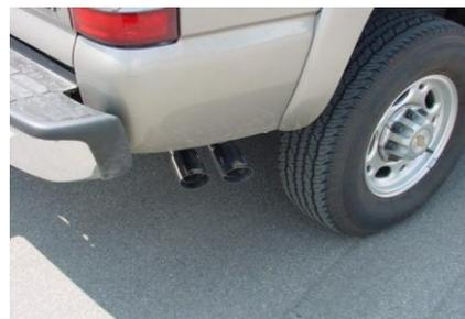
INSTALL YOUR BLACK CERAMIC COATED TIPS. PROCEED TO THE NEXT SHEET ON HOW TO INSTALL YOUR DEEGAN 38 BADGES. AFTER YOU HAVE CHECKED FOR CLEARANCES GO BACK AND TIGHTEN ALL NUTS, BOLTS AND CLAMPS.
