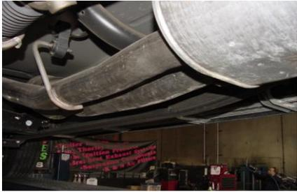
TO REMOVE STOCK EXHAUST, CUT 13" FROM THE FRONT OF THE MUFFLER, MEASURE TOWARDS THE FRONT OF THE VEHICLE. LEAVE ALL RUBBER GROMMETS ON THE HANGERS. USE WD-40 TO AID IN THE REMOVAL OF EXHAUST AND HANGERS. SUPPORT THE CATALYTIC CONVERTER BEFORE CUTTING.
