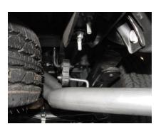
SLIDE PASSENGER SIDE TAILPIPE #E INTO OUTLET OF MUFFLER 1-1/2" TO 2". INSERT WELDED HANGER INTO RUBBER GROMMET. USE CLAMP #G TO SECURE TAILPIPE TO MUFFLER. DO NOT TIGHTEN.
