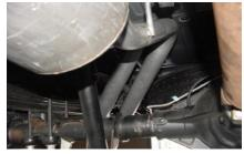
SLIDE DRIVERS SIDE TAILPIPE #D INTO MUFFLER 1-1/2" TO 2". GROMMET. USE CLAMP # J TO SECURE PIPE TO MUFFLER. DO NOT TIGHTEN. THE TAB ON THE TAILPIPE SHOULD BE ON THE TOP OF THE OTHER TAB,
