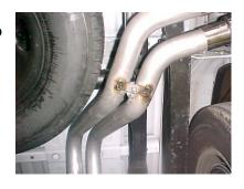
BOLT THESE TOGETHER USING BOLT KIT #H.
