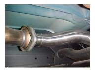
Install head pipe # A onto you're existing stock 2-bolt flange. Re-use your stock hardware to secure. Insert welded hanger into rubber grommet. Use a jack stand to support the converter. Do not tighten.
