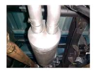
Install muffler onto head pipe #A 1-1/2" to 2" with the louvers facing towards the converter. Use a jack stand to support the muffler. Use clamp #H to secure the muffler to the head pipe. Do not tighten. Muffler inlet is looking into the louvers. The muffler outlets should be at the top.
