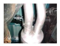
Install drivers side over axle tailpipe #C into muffler and secure pipe to muffler using clamp #G. Insert welded hanger into rubber grommet.
