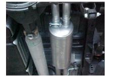
INSTALL MUFFLER #C ONTO HEADPIPES 1 ½" TO 2". USE CLAMP #G TO SECURE MUFFLER TO PIPES. DO NOT TIGHTEN. OUTLETS SHOULD BE AT THE TOP. SUPPORT MUFFLER WITH A JACK STAND.
