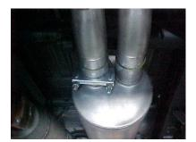
INSTALL REAR MUFFLER HANGER #H ONTO DRIVER SIDE OUTLET OF MUFFLER. INSERT HANGER INTO RUBBER GROMMET. DO NOT TIGHTEN.
