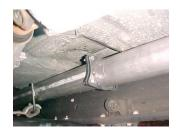
**INSTALL PIPE #B** ONTO PIPE #A. **USING GASKET AND BOLT KIT THAT IS** PROVIDED. INSERT WELDED HANGERS INTO RUBBER GROMMETS.
