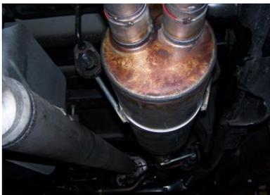
INSTALL MUFFLER #B ONTO HEADPIPE 1-1/2" TO 2". USE CLAMP #G TO SECURE THE MUFFLER TO THE HEADPIPE. DO NOT TIGHTEN. SLIDE BAND CLAMP #H ONTO THE MUFFLER AND INSERT THE WELDED HANGERS INTO THE RUBBER GROMMETS. ATTACH WITH BOLT KIT #J.
