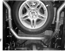
NEXT, INSTALL HANGER # G TO THE PASSENGER SIDE OF MUFFLER OUTLET WITH VERTICAL BAR OF THE HANGER TOWARDS PASSENGER SIDE INSTALL PASSENGER SIDE OVERAXLE PIPE # D INTO MUFFLER AT LEAST 1 ½" TO 2".AND USE CLAMP # F TO ATTACH.. DO NOT TIGHTEN
