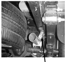
UNBOLT AND REMOVE STOCK REAR HANGER ON THE PASSENGER SIDEOF THE FRAME RAIL. INSTALL HANGERS # H TO THE BOTTOM OF FRAME RAIL IN EXISTING HOLE APPROX. 22 .5" FROM THE REAR OF THE FRAME, USE NUT AND BOLT THAT ARE SUPPLIED. REPEAT THIS SAME PROCEDURE ON DRIVERS SIDE. HANGER # H WILL AIM TOWARDS THE REAR OF THE VEHICLE.
