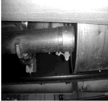
**DO NOT REMOVE THE EXTENSION PIPE BETWEEN THE MUFFLER AND THE CONVERTER.**
