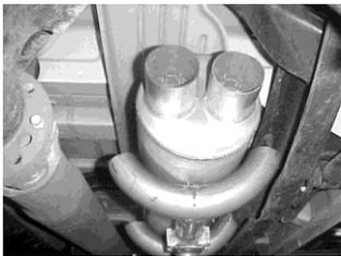
INSTALL MUFFLER ONTO STOCK HEADPIPE AND ATTACH WITH CLAMP #E. ALIGN NOTCH ON MUFFLER TO STOCK ALIGNMENT PIN ON FACTORY HEADPIPE. MUFFLER INLET IS TOWARDS THE CONVERTER. USE A JACK STAND TO SUPPORT THE MUFFLER.
