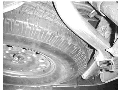
INSTALL DRIVER OVER AXLE TAILPIPE #C INTO MUFFLER 1-1/2" TO 2". INSERT WELED HANGER INTO RUBBER GROMMET. ROTATE PIPE UP UNTIL IT CONNECTS WITH REAR HANGER #F AND CONNECT TAILPIPE TO HANGER WITH CLAMP #E. **DO NOT TIGHTEN.**
