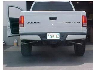
INSTALL YOUR STAINLESS STEEL TIPS. NOW GO BACK AND TIGHTEN ALL CLAMPS, NUTS AND BOLTS STARTING FROM THE FRONT AND WORK YOUR WAY BACK. USE ZIP TIES TO SECURE BRAKE LINES.
