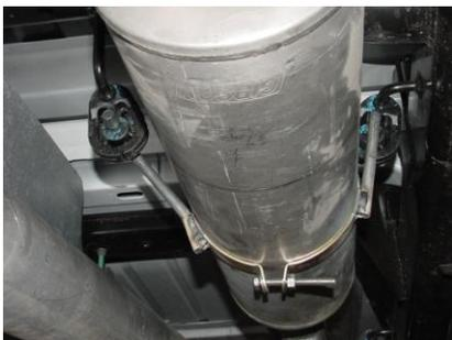
INSTALL MUFFLER #B ONTO HEADPIPE #A 1-1/2" TO 2". USE CLAMP #I TO SECURE THE MUFFLER TO THE HEADPIPE. DO NOT TIGHTEN. SLIDE BAND CLAMP #J ONTO THE MUFFLER AND INSERT THE WELDED HANGER INTO THE RUBBER GROMMET AND ATTACH TO MUFFLER WITH BOLT KIT #K.
