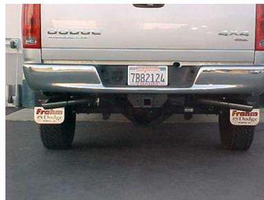
INSTALL THE STAINLESS TIPS. TO CLEAN TIPS USE ANY STAINLESS CLEANER AND A SCOTCH BRITE PAD. NOW GO BACK AND TIGHTEN ALL CLAMPS, NUTS AND BOLTS STARTING FROM THE FRONT AND WORKING BACK. USE ZIP TIES TO SECURE BRAKE LINE AWAY FROM EXHAUST.
