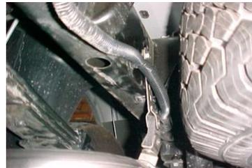
MEASURE 19 1/2" FROM THE REAR OF THE FRAME AND USE THIS HOLE AND BOLT ON HANGER #H ON THE INSIDE OF FRAME. USE THE 2<sup>ND</sup> HOLE FROM THE TOP.
