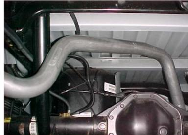
INSTALL DRIVER SIDE TAILPIPE #D INTO MUFFLER 1-1/2" TO 2" AND USE CLAMP #G TO SECURE TO THE MUFFLER. DO NOT TIGHTEN. USE CLAMP #G TO HOLD PIPE UP TO THE HANGER #H. DO NOT TIGHTEN.
