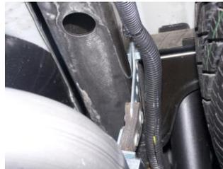
**5.** Use the hole 19 1/2" from the rear of the frame to attach the 10" hanger #F with bolt kit #M. Use the third hole from the top on the hanger.
