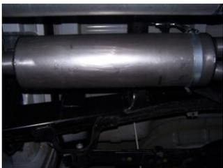
**3.** Install muffler #B onto head pipe #A 1 1/2"-2" with the louvers facing towards the converter. Use a jack stand to support the muffler. Use clamp #H to secure the muffler to the headpipe. Slide band clamp #I onto muffler and insert welded hangers into rubber grommets. Attach with bolt kit #K. DO NOT TIGHTEN. Muffler inlet is looking into the louvers.
