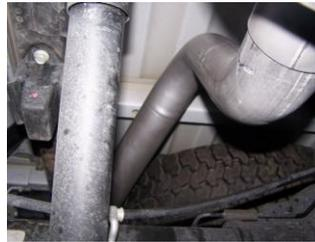
**4.** Install passenger side tailpipe #C into muffler 1 1/2"-2". Use clamp #G to secure tailpipe to muffler. DO NOT TIGHTEN. Insert welded hanger into rubber grommet.
