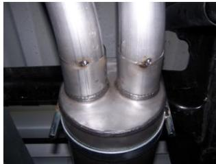
**6.** Install driver side tailpipe #D 1 1/2"-2" into muffler and use clamp #G to secure to muffler. Attach clamp #G to hold up to the hanger #F. DO NOT TIGHTEN.
