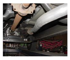
TO REMOVE STOCK EXHAUST UN-BOLT IT FROM THE 2-BOLT FLANGE LOCATED JUST BEHIND THE Y-PIPE. **DO NOT DAMAGE THE FACTORY HARDWARE, YOU WILL RE-USE IT.** NOW CUT OFF YOUR STOCK TAILPIPE JUST BEHIND THE MUFFLER AND REMOVE. LEAVE ALL RUBBER GROMMETS ON THE HANGER. USE WD-40 TO AID IN REMOVAL OF EXHAUST AND HANGERS.
