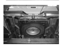
Install exit pipes # E onto the over axle pipes and attach with clamp #G. You may need to cut the exit pipes to your preference. Rotate all pipes until you have a minimum of a 1" clearance on all pipes. Use zip ties to reroute vent lines and brake lines. Tighten all clamps, flanges, bolts firmly. Stainless steel tips are optional.
