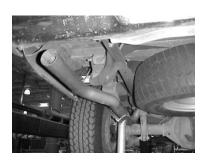
INSTALL THE EXIT PIPES #F TO YOUR DESIRED LOOK. ATTACH WITH CLAMP #G. MAKE SURE YOU HAVE A MINIMUM OF A 1" CLEARANCE FROM ALL BRAKE LINES, TIRES, SHOCKS FUEL LINES, ETC. THEN TIGHTEN ALL CLAMPS AND HANGERS. NOW INSTALL THE STAINLESS STEEL TIPS. USE SUPPLIED ZIP TIES TO TIE AWAY THE BRAKE AND FUEL LINES.
