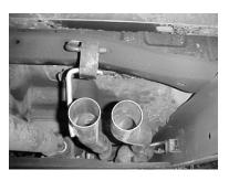
INSTALL HEADPIPE'S A & B. SLIP HEADPIPE #B'S WELDED HANGER INTO THE FACTORY RUBBER GROMMET. ROTATE HEADPIPE'S UNTIL THEY ARE POSITIONED DIRECTLY NEXT TO EACH OTHER. USE CLAMPS #J TO ATTACH THEM TO THE FACTORY HEADPIPE. DO NOT TIGHTEN
