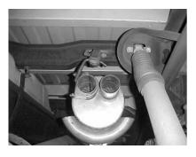
Slide muffler on 1-1/2" to 2" to headpipes and connect using clamps #G. DO NOT TIGHTEN. Level muffler outlets across at 12 o'clock position. Attach hanger #H to driverside muffler outlet and insert rod into rubber grommet.
