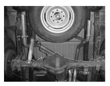
Install driver side over axle pipe #E. It will go in between shock and springs, above axle. Use hanger #H and clamp #G to attach to muffler. Attach clamp #G to hangers #I. Do not tighten. Pipes will be parallel to frame and out approximately ½". Use a level and tape measure to get both overaxle pipes the same.
