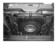
Now install exit pipes #F to tailpipe using clamp #G. Trim Exit Pipes to desired length. Now tighten all clamps down starting from the head pipe and working back. Re-route vent line, and tie back brake lines with zip ties. Install Stainless tips
