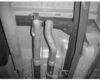
Slide head pipes #A or B over stock headpipes 1-1/2" to 2". Insert welded hanger on driver side headpipe into rubber grommet. Attach headpipe to stock headpipe with clamps #J.
