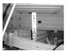
Remove stock rear tailpipe hanger. Measure 25-1/2" from the rear of the frame, you will see a 3/8" hole, use this hole to bolt up hangers #I. You will use the third hole down from the top of the hanger.
