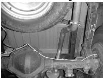
Insert passenger side overaxle pipe #D 1-1/2" to 2" and attach to muffler with clamp #G. Do not tighten.
