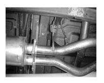
INSTALL MUFFLER # C WITH THE OUTLETS OF THE MUFFLER POSITIONED AT THE TOP USE A JACK STAND TO SUPPORT MUFFLER. INSTALL CLAMPS # H AT THE INLETS OF THE MUFFLER AND ATTACH TO HEADPIPE. (DO NOT TIGHTEN). ATTACH HANGER # I TO THE REAR OF THE MUFFLER ON THE DRIVER SIDE OUTLET. (DO NOT TIGHTEN).
