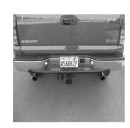
WHEN YOU HAVE EVERYTHING IN PLACE FIRMLY TIGHTEN ALL CLAMPS AND HANGERS. YOU MAY NEED TO USE THE SPARE TIRE BRACKET TO HOLD THE TIRE BACK. INSTALL IT 2" INSIDE OF THE UPPER SHOCK MOUNT ON THE DRIVER SIDE. USE ZIP TIES TO TIE AWAY BRAKE LINES. RE-INSTALL THE O2 SENSOR INTO PASSENGER HEADPIPE. USE ANTI-SEIZE ON ALL THREADS. INSTALL STAINLESS TIPS.
