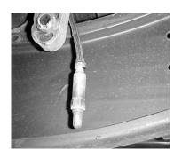
UN-BOLT THE FACTORY 02 SENSOR BEHIND THE PASSENGER CATALYTIC CONVERTER (CAREFULLY REMOVE SO NO DAMAGE OCCURS!) REMOVE THE FACTORY EXHAUST BY CUTTING 16" IN FRONT OF THE MUFFLER ON THE PASSENGER SIDE AND UN-BOLT 33" IN FRONT OF YOUR MUFFLER ON THE DRIVER SIDE HEADPIPE. FOR EASIER REMOVAL OF THE STOCK EXHAUST YOU MAY NEED TO CUT YOUR STOCK TAILPIPE BEHIND THE MUFFLER. MAKE SURE TO LEAVE ALL STOCK RUBBER MOUNTING GROMMETS IN PLACE. USE WD-40 ON ALL RUBBER GROMMETS.
