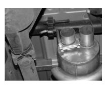
INSTALL MUFFLER #B ONTO HEADPIPE AT LEAST 1½" TO 2". USE CLAMP #F TO SECURE MUFFLER TO HEADPIPE. DO NOT TIGHTEN. USE A JACK STAND TO SUPPORT THE MUFFLER. OUTLETS SHOULD BE AT THE TOP. INSTALL HANGER #I ONTO DRIVERSIDE MUFFLER OUTLET AND INSERT WELDED HANGER INTO GROMMET. DO NOT TIGHTEN.
