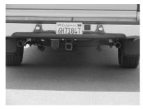
INSTALL EXIT PIPES #E ONTO TAILPIPES. CUT TO YOUR PREFERED LENGTH USE CLAMPS #G TO SECURE EXIT PIPES TO TAILPIPES. THESE CLAMPS ALSO ATTACH TO METAL HANGERS #H. THESE METAL HANGERS NEED TO BE ROTATED IN ORDER TO ADJUST FOR CLAMPING. NOW YOU CAN TIGHTEN ALL CLAMPS, NUTS, AND BOLTS. STARTING FROM THE FRONT WORKING BACK. USE ZIP TIES TO TIE AWAY BRAKE LINES. INSTALL STAINLESS TIPS.
