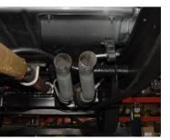
INSTALL PASSENGER SIDE OVER AXLE TAILPIPE #E INTO MUFFLER 1 ½" TO 2" INSERT WELDED HANGER INTO RUBBER GROMMET. USE CLAMP # J TO SECURE PIPE TO MUFFLER. DO NOT TIGHTEN.
