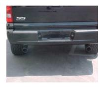
TAILPIPES, CUT TO YOUR PREFERED LENGTH USE CLAMPS # I TO SECURE EXIT PIPES TO TAILPIPES. THESE CLAMPS ALSO ATTACH TO METAL HANGERS # J. THESE METAL HANGERS NEED TO BE ROTATED IN ORDER TO ADJUST FOR CLAMPING. NOW YOU CAN TIGHTEN ALL CLAMPS, NUTS, AND BOLTS. STARTING FROM THE FRONT WORKING BACK, INSTALL STAINLESS TIPS. USE ZIP TIES FOR BRAKE AND FUEL LINES.
