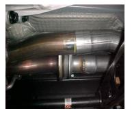
INSTALL PASSENGERSIDE HEADPIPE #A ONTO FACTORY FLANGE USING THE HARDWARE # K. DO NOT TIGHTEN. INSERT HANGER INTO RUBBER GROMMET, NEXT, INSTALL DRIVERSIDE HEADPIPE #B ONTO THE FACTORY PIPE. USE CLAMP # I TO SECURE. DO NOT TIGHTEN.
