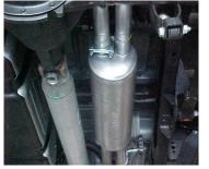
INSTALL MUFFLER #C ONTO HEADPIPES 1 1/2" TO 2". USE CLAMP #G TO SECURE MUFFLER TO HEADPIPES. DO NOT TIGHTEN. OUTLETS SHOULD BE AT THE TOP. SUPPORT MUFFLER WITH A JACK STAND.
