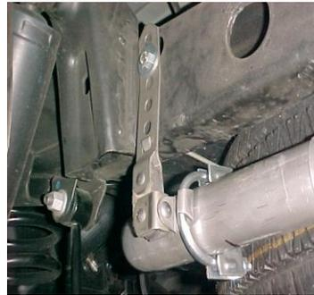
INSTALL METAL HANGER # I INTO HOLE LOCATED APPROXIMATELY 23" FROM THE REAR OF THE FRAME. USE TOP HOLE ON HANGER. INSTALL DRIVER SIDE OVERAXLE TAILPIPE # C INTO THE MUFFLER 1-1/2"-2". USE CLAMP #H TO SECURE PIPE TO MUFFLER.DO NOT TIGHTEN.
