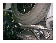
INSTALL DRIVERS SIDE OVERAXLE TAILPIPE # D INTO MUFFLER 1-1/2" TO 2". ATTACH TO MUFFLER OUTLET USING CLAMP #I INSERT WELDED HANGERS INTO RUBBER GROMMETS. DO NOT TIGHTEN.
