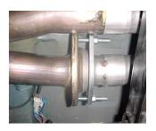
BOLT PASSENGER SIDE HEADPIPE # A ONTO FACTORY DOME USING HARDWARE KIT # L. DO NOT TIGHTEN. INSERT HANGER INTO RUBBER GROMMET, NEXT SLIP DRIVER SIDE HEADPIPE # B ONTO FACTORY PIPE USE CLAMP # H TO SECURE. DO NOT TIGHTEN.
