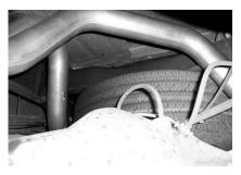
INSTALL PIPE #A ONTO TURBO. SECURE TURBO USING FACTORY CLAMP. INSERT WELDED HANGER INTO RUBBER GROMMET. SNUG TURBO CLAMP BUT **DO NOT TIGHTEN**
