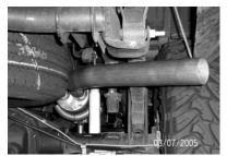
INSTALL PASSENGERSIDE EXIT PIPE #F ONTO
