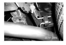
INSTALL PIPE #B ONTO DOWN PIPE #A. USING GASKET #J AND BOLT KIT # I. INSERT WELDED HANGER INTO RUBBER GROMMET.
