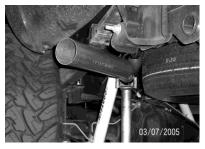
INSTALL DRIVERSIDE EXIT PIPE #G ONTO TAILPIPE. USE CLAMP #L TO SECURE TOGETHER. DO NOT TIGHTEN. INSERT WELDED HANGER INTO RUBBER GROMMET ROTATE TO THE BEST FIT FOR YOUR VEHICLE.
