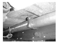
BOLT HEADPIPE #A ONTO FACTORY 4-BOLT FLANGE USING SUPPLIED BOLT KIT #H AND GASKET #I. BEFORE YOU INSTALL MUFFLER INSTALL BAND CLAMP HANGER #L
