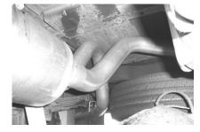
INSTALL DRIVERSIDE OVERAXLEPIPE # D INTO MUFFLER 1 ½"-2". USE CLAMP #K TO SECURE PIPE TO MUFFLER OUTLET. **DO NOT TIGHTEN**
