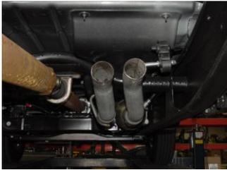
**3.** SLIDE PASSENGER SIDE HEADPIPE #A ONTO STOCK HEADPIPE. INSERT WELDED HANGER INTO RUBBER GROMMET. NEXT INSTALL DRIVERS SIDE HEADPIPE # B, AND USE CLAMP #I TO SECURE BOTH HEADPIPES. DO NOT TIGHTEN.
