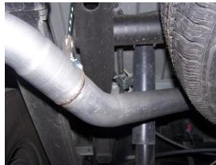
**8.** INSTALL DRIVER SIDE OVER AXLE TAILPIPE #D INTO THE MUFFLER. 1½" TO 2" ROTATE PIPE UNTIL IT HITS THE 10" HANGER USE CLAMP # K TO HOLD UP THE PIPE. ATTACH TAILPIPE TO MUFFLER USING CLAMP # H. DO NOT TIGHTEN.
