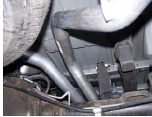
**7.** INSTALL PASSENGER SIDE OVER AXLE TAILPIPE #E INTO MUFFLER 1½" TO 2" INSERT WELDED HANGER INTO RUBBER GROMMET. USE CLAMP # J TO SECURE PIPE TO MUFFLER. DO NOT TIGHTEN.
