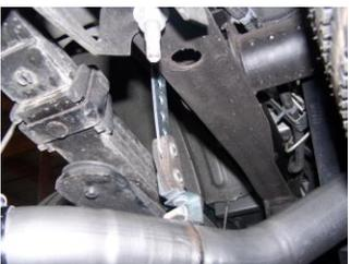
**6.** MEASURE 18" FROM THE REAR OF THE FRAME TOWARDS THE FRONT OF THE VEHICLE. USE THIS SLOT FOR THE 10" HANGER #K, INSTALL USING THE 1<sup>ST</sup> HOLE USE HARDWARE KIT #L.
