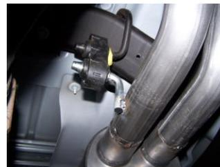
Bolt head pipe #A onto your existing stock front pipe re-using stock nuts/bolts. Insert welded hanger into rubber grommet. DO NOT TIGHTEN.
