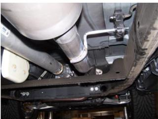
**4.** Install muffer #B onto head pipe #A 1½"-2". Muffer outlets will be positioned at the top. Use a jack stand to support the muffer. Use clamp #E to secure the muffer to the headpipe. DO NOT TIGHTEN.
