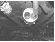
**4.)** SLIP TAILPIPE #C INTO THE PASSENGER SIDE OUTLET NO MORE THEN 2" AND NO LESS THEN 1". THEN SLIP THE WELDED HANGER INTO THE FACTORY RUBBER GROMMET. USE CLAMP # G TO TIGHTEN THE CONNECTION AT THE MUFFLER OUTLET. DO NOT TIGHTEN CLAMPS.
