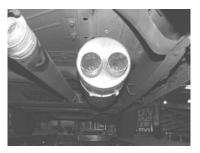
3.) SLIP MUFFLER # B ONTO HEADPIPE #A NO MORE THEN 2" AND NO LESS THEN 1" WITH THE INLET TOWARDS THE MOTOR. USE A JACK STAND TO SUPPORT THE MUFFLER. MAKE SURE THE MUFFLER OUTLETS ARE LEVEL. DO NOT TIGHTEN
