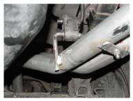
5.) SLIP TAILPIPE #D INTO THE DRIVER SIDE OUTLET NO MORE THEN 2" AND NO LESS THEN 1". USE HANGER #G TO TIGHTEN THE CONNECTION AT THE MUFFLER OUTLET. DO NOT TIGHTEN. TOWARDS THE END OF THE PIPE THERE IS A TAB USE BOLT KIT #H TO SECURE PIPES TOGETHER. DRIVERSIDE GOES ON THE BOTTOM.
