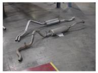
1.) TO REMOVE EXHAUST-UNBOLT IT FROM THE 2 BOLT FLANGE LOCATED JUST BEHIND THE CATALYTIC CONVERTER. YOU WILL RE-USE THESE BOLTS. NOW CUT OFF YOUR STOCK TAILPIPE JUST BEHIND THE MUFFLER AND REMOVE. LEAVE ALL RUBBER GROMMETS ON THE HANGERS. USE WD-40 TO AID IN REMOVAL OF EXHAUST AND HANGERS.
