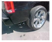
"MAKE SURE HAVE A MINIMUM OF A 1" ON ALL PIPES FROM ALL RUBBER BRAKE LINES, TIRES, SHOCKS, FUEL LINES, ETC."
