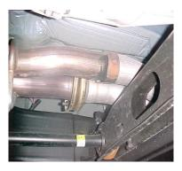
TO REMOVE STOCK EXHAUST CUT YOUR STOCK TAILPIPE OFF, REMOVE HANGERS FROM RUBBER GROMMETS, USE WD-40 TO HELP WITH REMOVAL. NOW UN-BOLT YOUR FACTORY EXHAUST AT THE FLANGE LOCATED JUST AFTER YOUR Y-PIPE.
