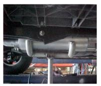
NEXT INSTALL MUFFLER #C. SLIDE IT ONTO HEADPIPE 1-1/2" TO 2". INLET OF MUFFLER SHOULD FACE TOWARDS THE MOTOR. ATTACH TO HEADPIPE WITH CLAMP #G. INSTALL REAR MUFFLER HANGER #J INTO RUBBER GROMMET LOCATED JUST ABOVE THE DRIVERS SIDE OUTLET OF THE MUFFLER. SLIDE CLAMP ONTO MUFFLER OUTLET. INLET OF MUFFLER IS
