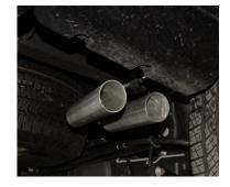
INSTALL DRIVERS SIDE OVERAXLE TAILPIPE #E INTO MUFFLER 1-1/2" TO 2". ATTACH TO MUFFLER WITH HANGER #J. USE BOLT KIT #K TO ATTACH BOTH TAILPIPES TOGETHER. DRIVERS SIDE TAB WILL BE ON THE BOTTOM.
