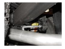
INSTALL PASSENGER SIDE OVERAXLE TAILPIPE #D INTO MUFFLER 1-1/2" TO 2". INSERT WELDED HANGER INTO RUBBER GROMMET. USE CLAMP #I TO SECURE PIPE TO MUFFLER. DO NOT TIGHTEN.
