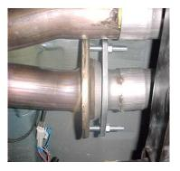
BOLT HEADPIPE # A ONTO STOCK HEADPIPE AND ATTACH TO FLANGE WITH BOLT KIT #L. INSERT WELDED HANGER INTO RUBBER GROMMETT. DO NOT TIGHTEN. INSTALL HEADPIPE # B, SLIP IT ONTO THE STOCK HEADPIPE USING CLAMP # G TO SECURE THE HEADPIPE TO THE STOCK PIPE. DO NOT TIGHTEN.
