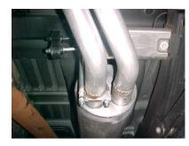
"MAKE SURE YOU HAVE A 1" CLEARANCE ON ALL PIPES FROM BRAKE AND FUEL LINES, TIRES, SHOCKS, ETC..."
